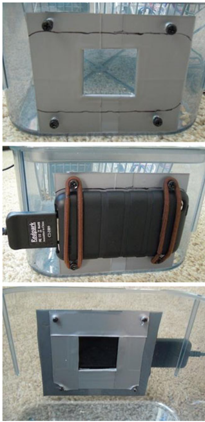
Fig. 3 Top panel: Close-up view of the opening on the front wall of the plastic box, which fits the area of the screen of the iPod Touch containing the button that will present stimuli and detect/register responses from the animal during training (i.e., the response key). Middle panel: Same view, now with the iPod Touch already mounted on the wall. Bottom panel: View from inside the box. As can be appreciated, only a small portion of the screen of the iPod Touch will be visible and accessible to the animal
