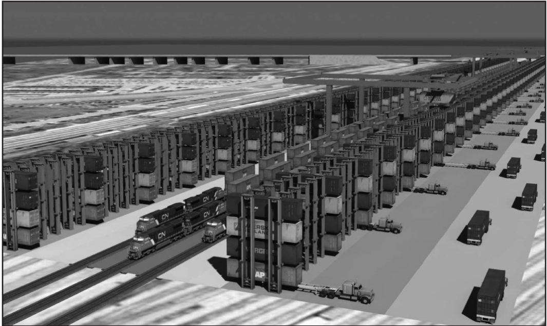
Figure 5: A Ramp With Vertical ATMS Stations
