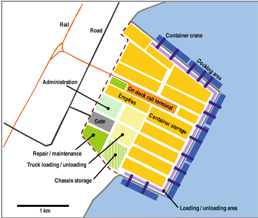
Fig. 49.4 Port container terminal facility. (Source: Author)
